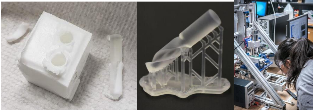
RET participants create drill bits with different helix and point angles and test the force and torque that occurred.
