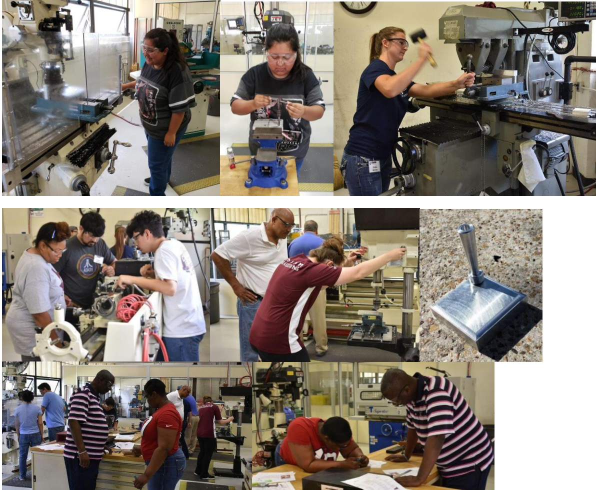
RET participants using aluminum stock to create a finished pen base and pen holder on sawing machines, horizontal mill, vertical mill, drill press, lathe, and taps.
