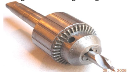
Fig. L4.8. Fixed center-drill and chuck (at tailstock)
