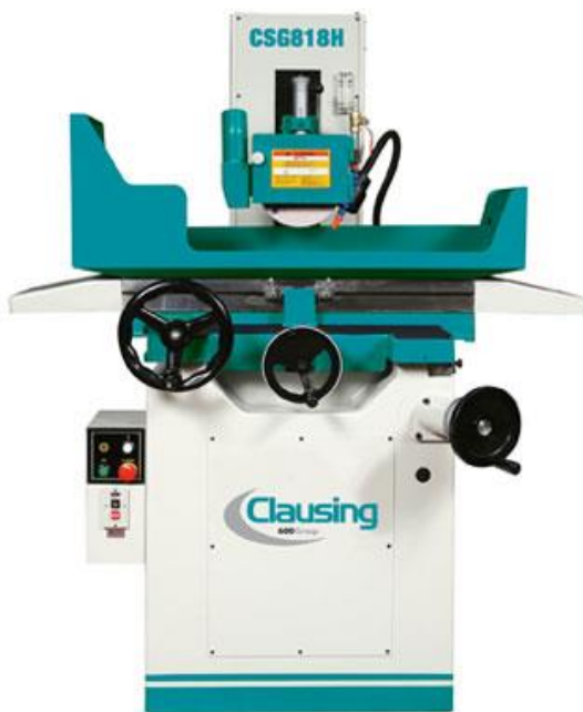
Fig L4.21. Clausing CGS 818H surface grinder
