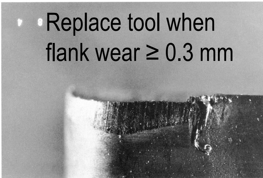
Flank wear (side view)
