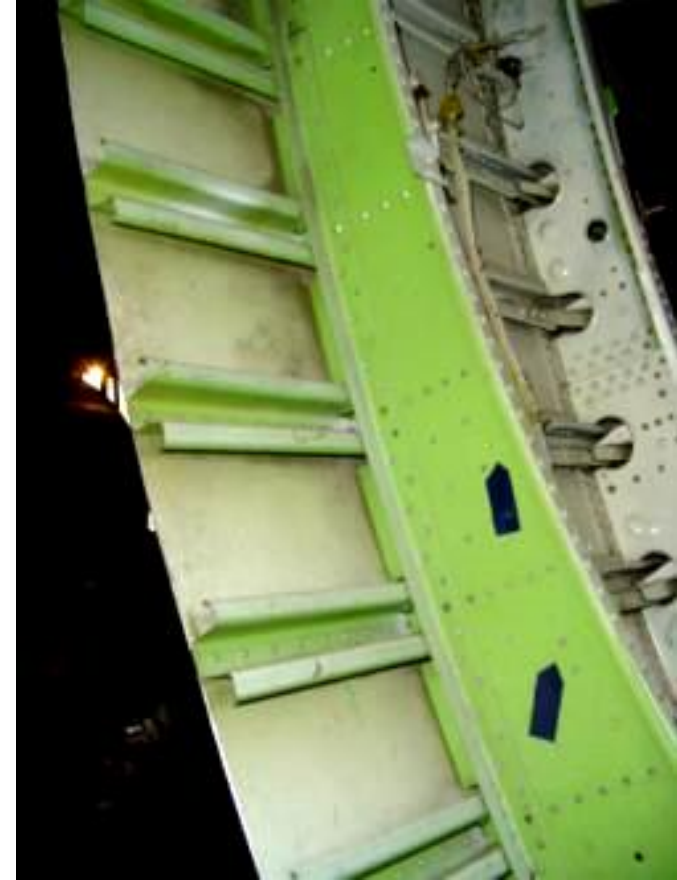
Aluminum fuselage of a Boeing 747 Source: http://en.wikipedia.org/wiki/Fuselage
