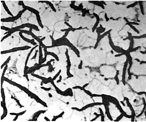
Gray cast iron with graphite flake
