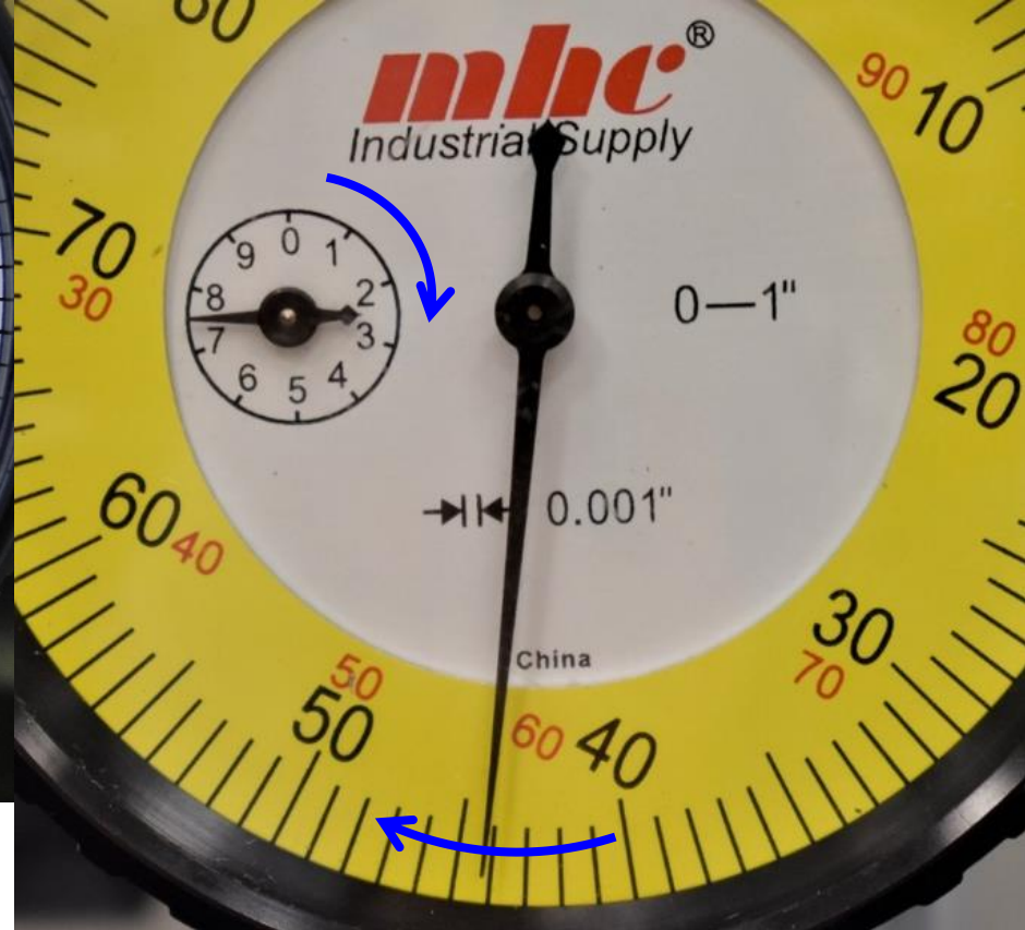
MHC indicator with long and short hands rotate in same directions
