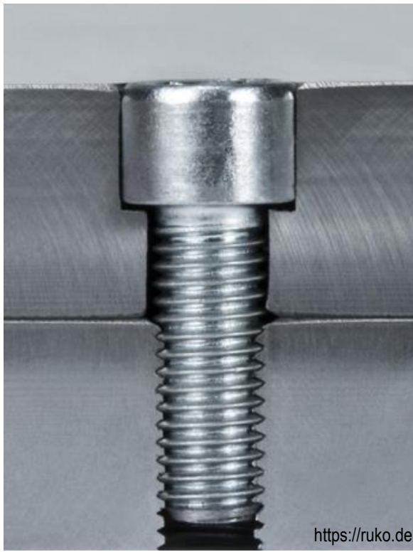
Counter bored hole for cylindrical screw head
