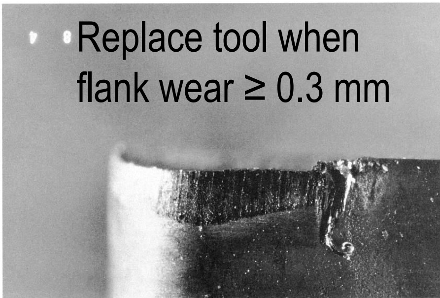
Flank wear (side view)
