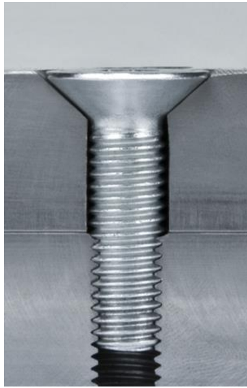
Counter sunk hole for conical screw head
