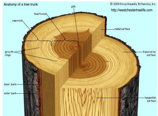
Wood is anisotropic. Its strength depends on loading directions (along or across the grains), or content of moisture /chemical treatment.
